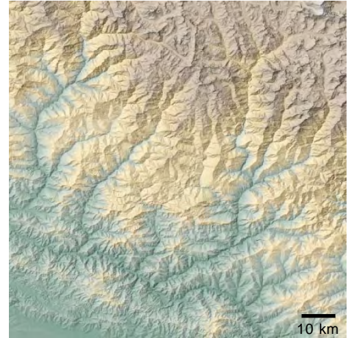
ASTER Global DEM tile N27E086, Nepal. This tile spans the foothills and crest of the Himalaya Mountains. The topographic complexity in this tile results in less efficient JPEG2000 compression (see table below).
