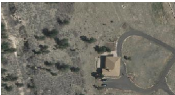
Orthoimage (left) and relief-shaded virtual surface (right) constructed in the TNT view from LAS LIDAR points of a small area (165 meters across) outside Denver, Colorado. The scene includes a house, driveway, and scattered trees. LIDAR points covering this area (shown in illustration below left) have a spacing of 50 to 70 centimeters. Bare-earth points have been classified by the vendor using an automated procedure, leaving remaining points unclassified. The virtual surface is based on both bare-earth and unclassified points, so the house and trees are clearly visible in the virtual surface along with natural topographic features. See the Technical Guide entitled LIDAR: View LAS Point Cloud as Surface for details on virtual surface display.
