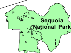
Vector object with park boundary and subarea polygons. Extract Tileset automatically determines the outer boundary of the contiguous polygons to define the clipping area.
